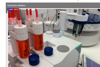
Experiment 1: Remote autotitrator for an acid-base titration.
